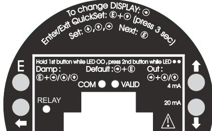
**Procedure of programming:** press button in the relevant sequence and check the state of the LED-s. Symbols for the states of the LED-s:
