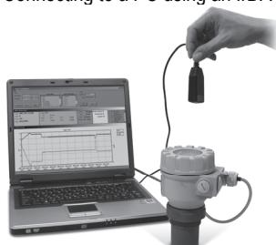
The IrDA adapter and the IrDA port of the device must be placed whithin a 5...10 cm distance and facing each other!
