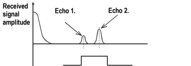
Some applications involve multiple (target + disturbing) echoes even within the measuring window. Basic echo selection will be done by the Quest + software automatically. This parameter only influences the echo selection within the measuring window.
