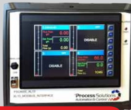
Capable of controlling 4 mini CORI-FLOW or more if needed
