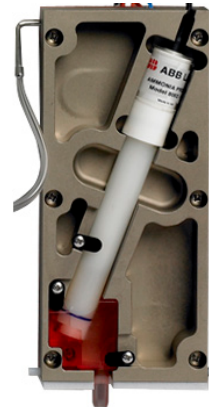
Figure 3 Electrode in temperature-controlled flow cell
