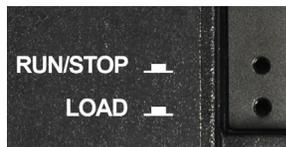
Two recessed buttons provide control of several RCC modes. A paperclip may be used as the buttons are far enough recessed that a pen or pencil is not able to activate them.
