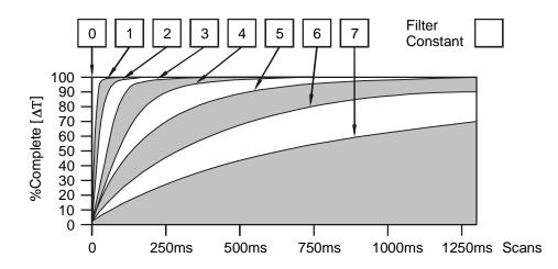
*Digital Filtering*. The illustration above demonstrates the effect of digital filtering (set with Filter Constant) on module response to a temperature change.
