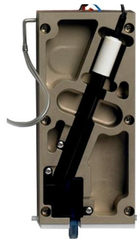
Figure 3 Electrode in temperature-controlled flow cell
