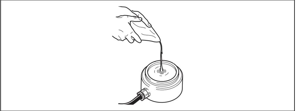
Fig. 4.2 Potting the Terminal Box – WaterMaster FET1 Transmitter
